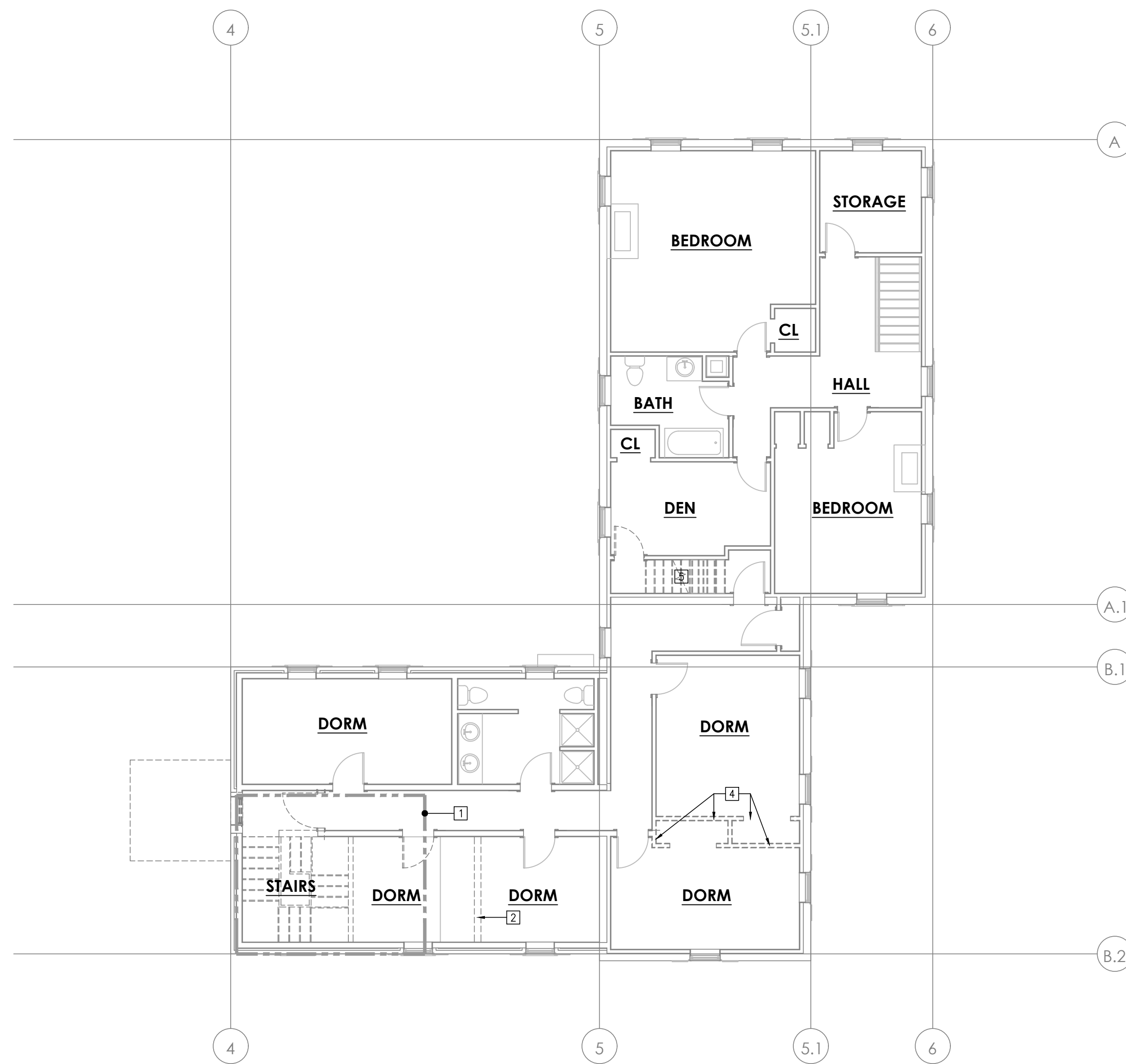
ELECTRICAL DEMOLITION SECOND FLOOR SCALE: 1/8"=1'-0"
