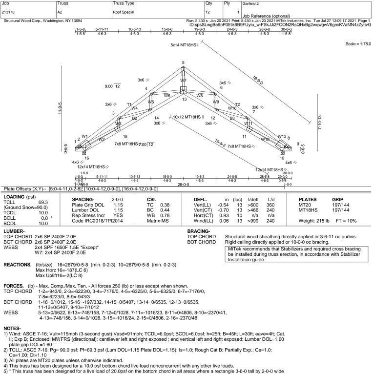
5) \* This truss has been designed for a live load of 20.0psf on the bottom chord in all areas where a rectar will fit between the bottom chord and any other members.
