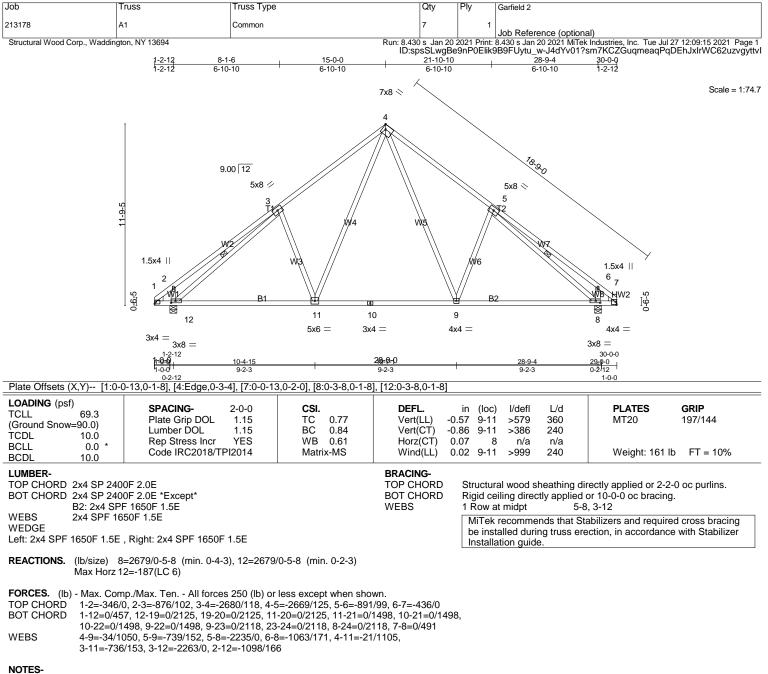
Wind: ASCE 7-16; Vult=115mph (3-second gust) Vasd=91mph; TCDL=6.0psf; BCDL=6.0psf; h=25ft; B=45ft; L=30ft; eave=4ft; Cat. II; Exp B; Enclosed; MWFRS (directional); cantilever left and right exposed ; end vertical left and right exposed; Lumber DOL=1.60 plate grip DOL=1.60
