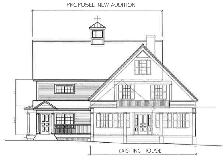
1 PROPOSED SOUTH ELEVATION Scale: 1/8" = 1'-0"
