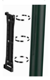
**Step 2:** secure the radar to the bar and lock it into place (optional) (pad lock not included)
