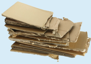
Corrugated Cardboard (Wavy center layer)
