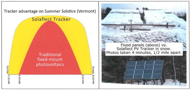
Over the course of the year, the Tracker produces about 40% more energy than an equivalent fixed-mount solar array. Fuller use of long summer days and automatic shedding of snow are two reasons for this increase in productivity.
