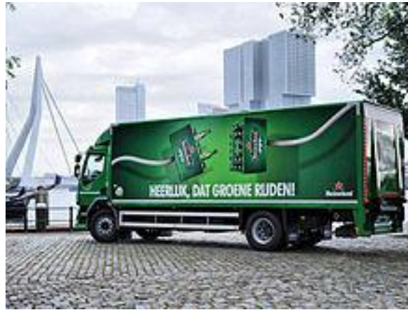
2013: Dutch Emoss 19-ton truck, 200 mile range 7 other Dutch electric trucks in operation
